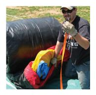
**Step 7**: Where the Inflatable roll is to end- tuck in rope or strap 60-90 cm underneath Inflatable that is to be used for tying. (Doing so will allow you to not lift the entire roll to tie off.)
